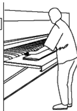
Figures 10 - Retrieving small pieces of laundry from the rolling ironer
